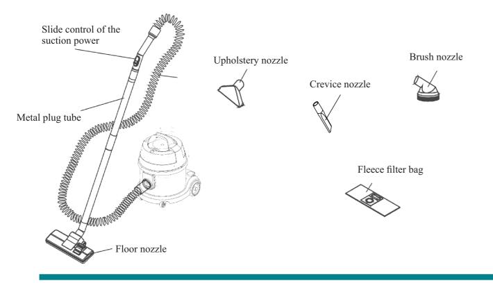
The flexible suction hose with rotating end pieces facilitates the operation of the accessories. The bleed valve is on the handle of the suction hose.
