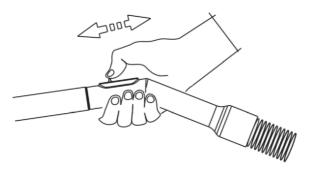
Connect the metal tube with the handle of the suction hose and the accessory to the pipe.
